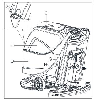
switch (F). If necessary, the forward speed can be adjusted with the adjuster (H).
